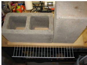
We used two bricks to bend shelves.
